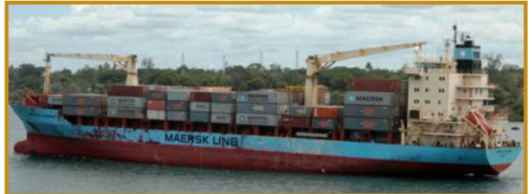
"MV Maersk Alabama" (Voir Web maritime p.9 - "Captain Phillips") 155m. x 25,30m. - DWT 17375 - 1092 TEU
