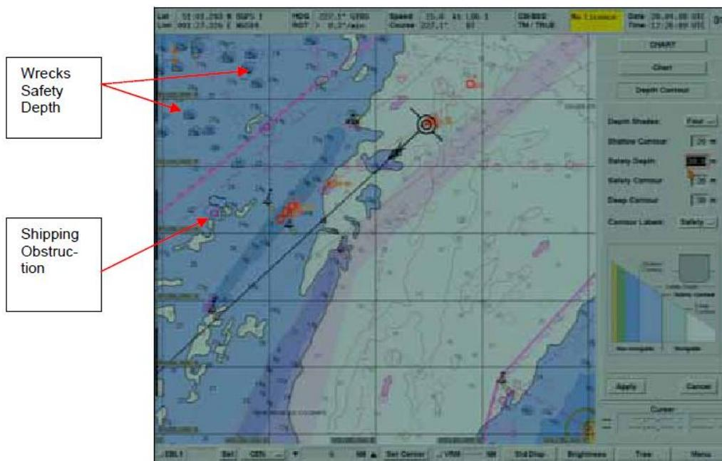
The safety depth in the picture above is set to 30 meters and the chart is in day mode displaying four colours. The sand bank is identifiable as dark blue, it is still behind the safety contour as it is set to 30 meters and thus does not stand out.
